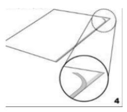
Unfold the PVC foil on a table. Remove the double-sided tape.
