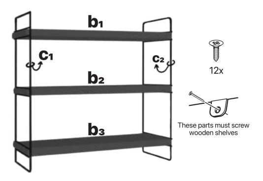
**Note:** Use the screws for fitting the wood shelf to **the metal frame** at screw plates.
