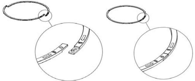
The part "5-3" is locked from the double-sided locking mechanism as in "Figure D"
