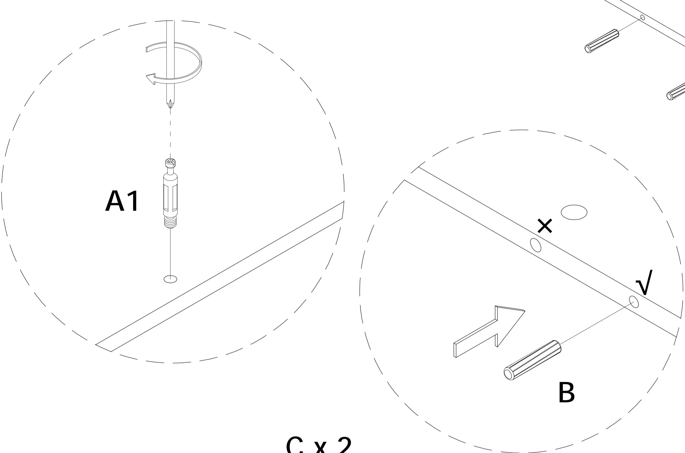
Hint: When installing, please make sure the screws are flattened, Not crooked; Otherwise the drawers will not be installed perfectly.
