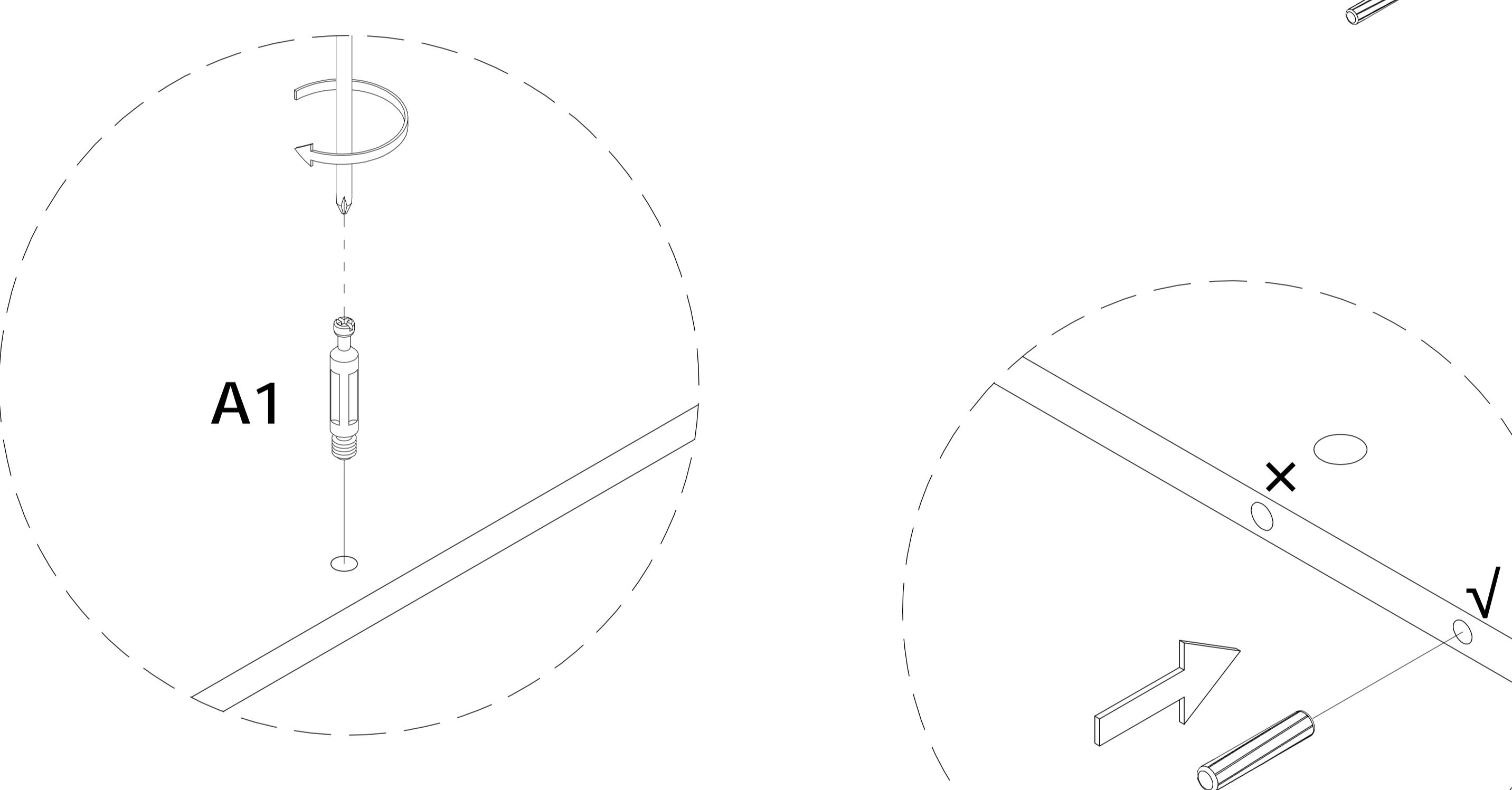
Hint: When installing, please make sure the screws are flattened, Not crooked; Otherwise the drawers will not be installed perfectly.
